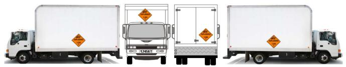
**Example:** The placard is to be displayed on all sides of the vehicle.
