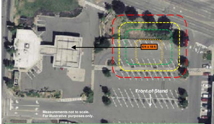
**Required Distances Away From A Retail Fireworks Stand** Green Line = No Parking or motor vehicle traffic on public road, 20 feet = 30 feet from tent; No combustable vegitation and waste material **Red Line** = No buildings or combustibles, 40 feet from front, 20 feet from sides. = Property line; 5 feet from back and sides, 20 feet to front. Black Line = Retail fireworks stand shall not be closer than 100 feet from a vehicle dispensing station.
