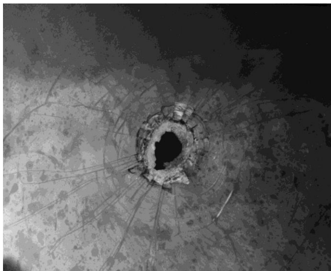
Photograph of cratering on the exit side of the windshield.
