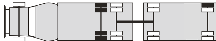
All tires on one drive axle and one tire on either side of last trailer axle.
