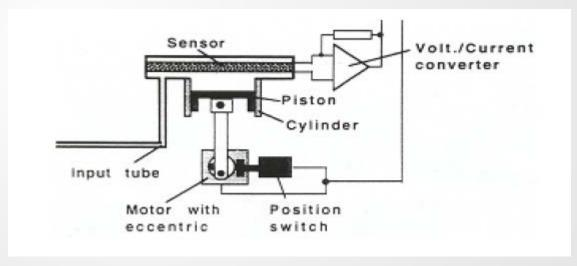
**Electrochemical Sensor (Fuel Cell)**
